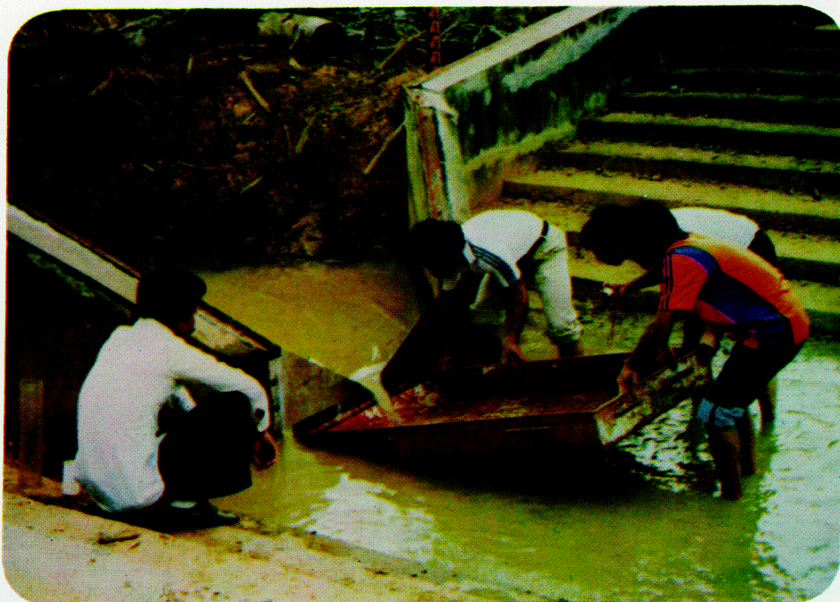
PLATE3.3—A TYPICAL GAUGING STATION (CALIBRATION BY VOLUMETRIC METHOD IN PROGRESS)
