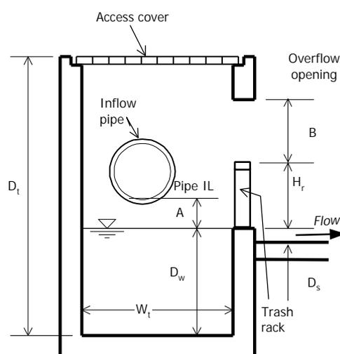
Figure 34.7 GPT Type 2 Trap Dimensions
