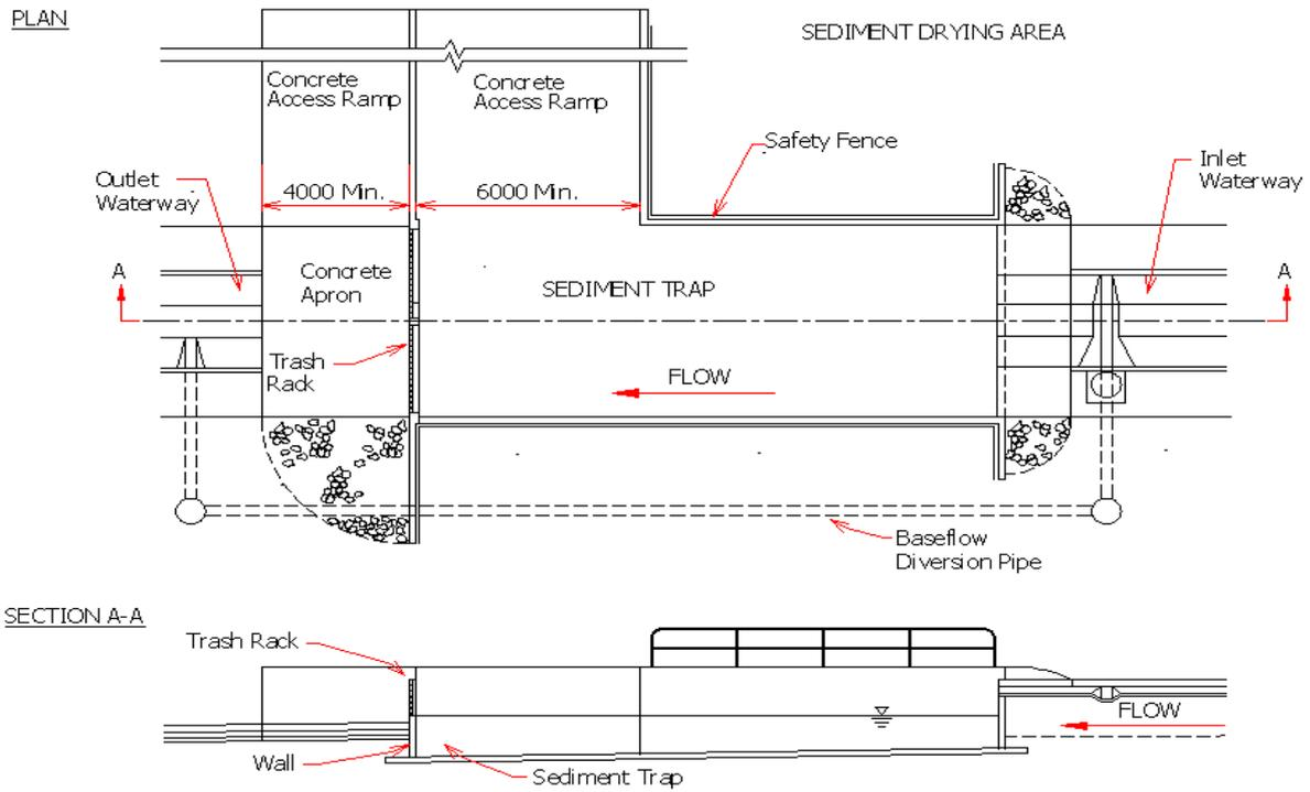
Figure 34.4 Type 1 SBTR Trap Configuration
