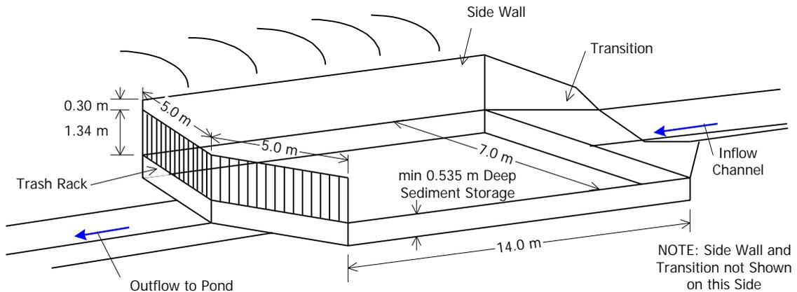
Figure 34.D1 Diagrammatic Layout of Proposed Type 1 SBTR Trap for Sg. Rokam example
