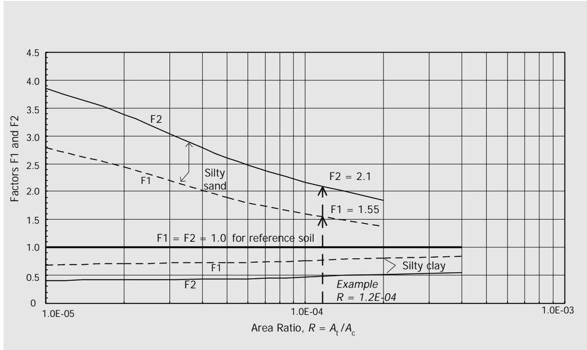
Design Chart 34.A2 Soil Type Adjustment Factors for Trap Area and Sediment Volume
