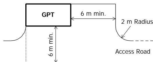
Figure 34.9 Access Requirements for SBTR Trap Type 2 (source: ACT City Services, 1994)
