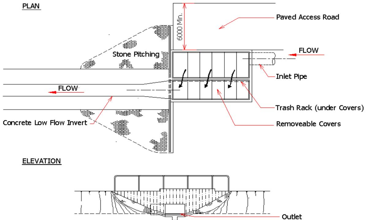
Figure 34.5 Type 2 SBTR Trap Configuration
