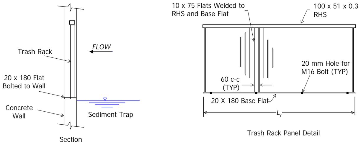
Figure 34.8 Typical Trash Rack for SBTR Trap
