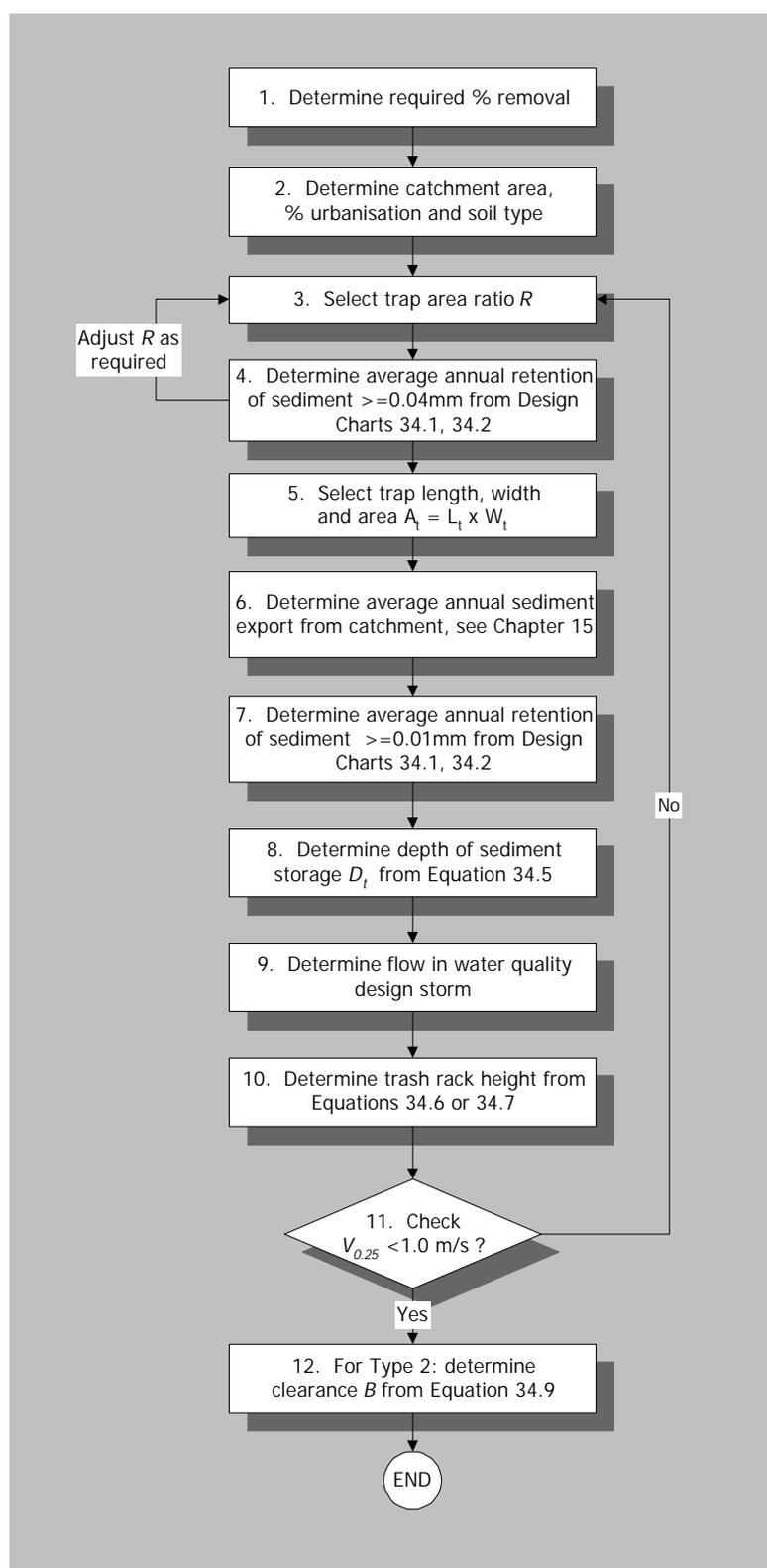
Figure 34.6 Flowchart for SBTR Trap Size Calculation
