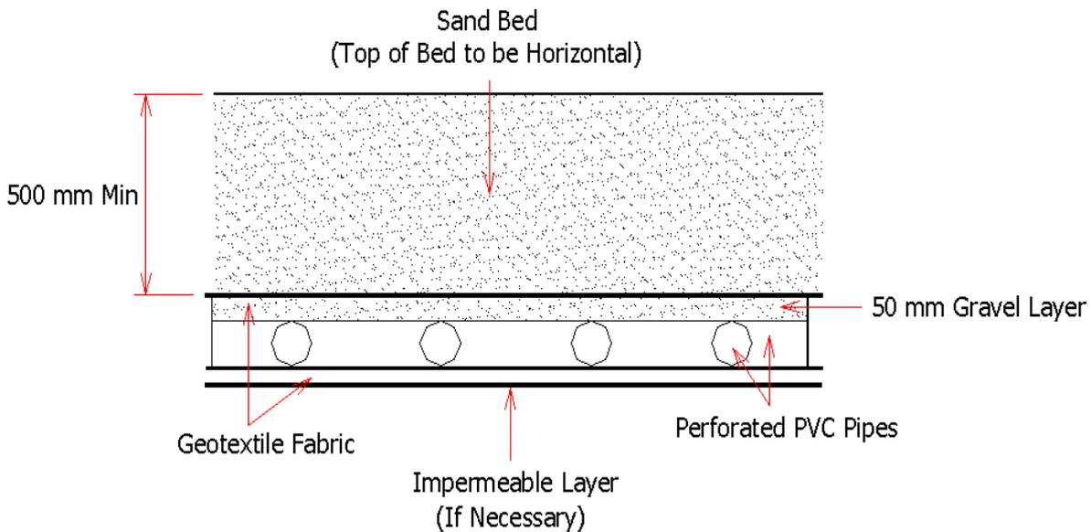
Figure 31.8 Sand Bed Profile with Gravel Layer
