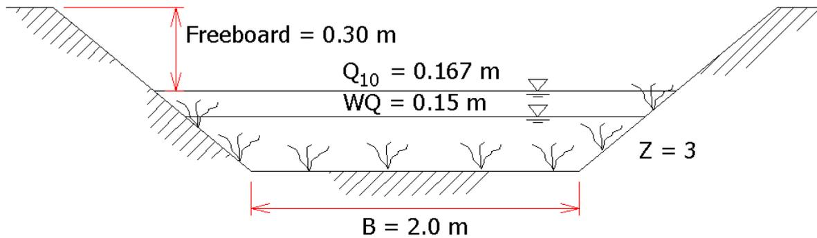
Figure 31.A2 Swale Designed Section
