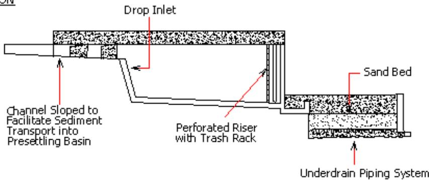
Figure 31.6 Sand Filtration Basin Preceded By Presettling Basin
