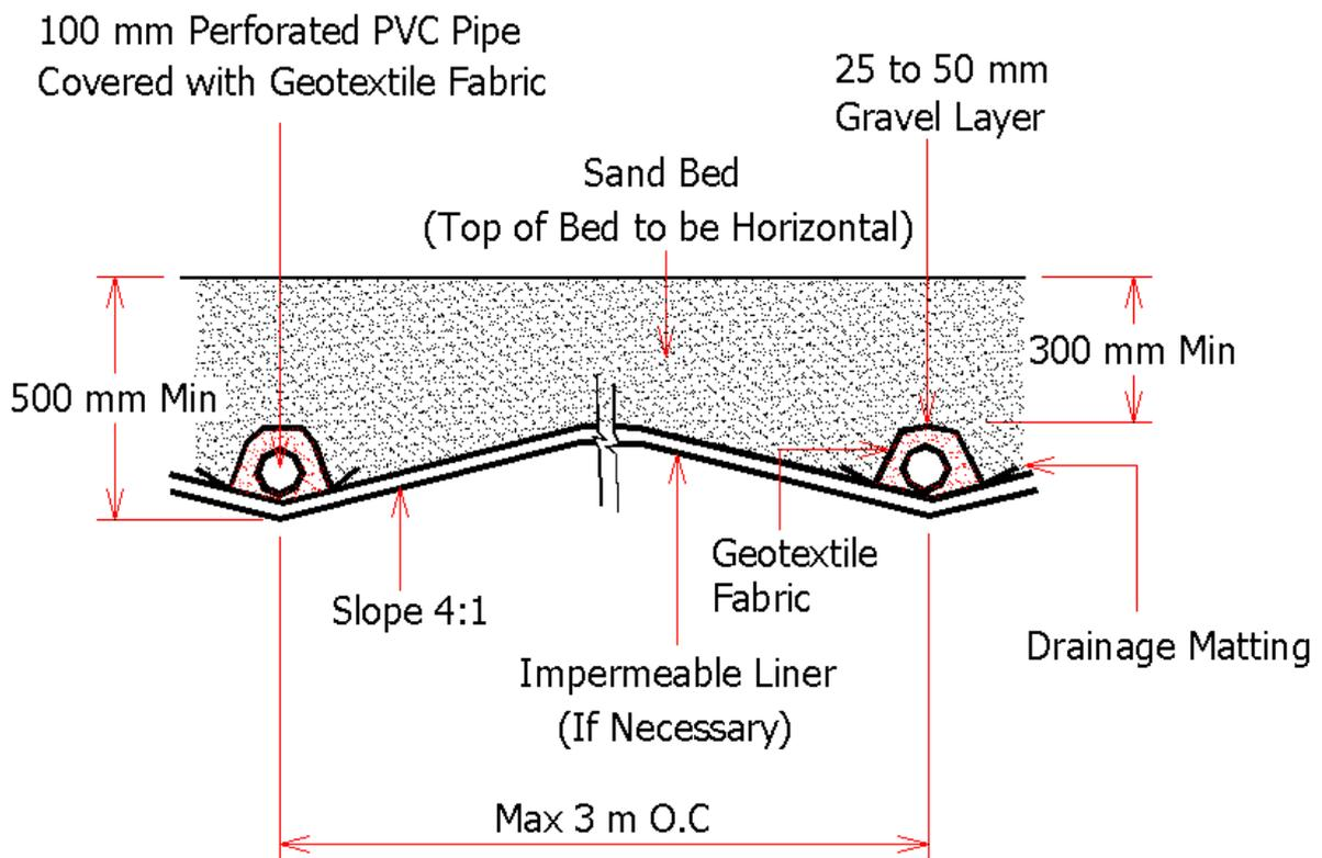
Figure 31.9 Sand Bed Profile with Trench Design (Source : City of Austin, 1988)
