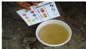
Pemantauan Parameter (pH, coliform, turbidity, dissolved oxygen, phosphate, nitrate) Kualiti Air Guna Test Kit
