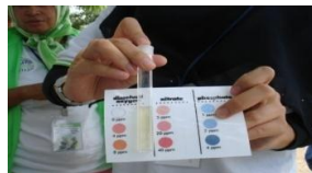
Pemantauan Parameter (pH, coliform, turbidity, dissolved oxygen, phosphate, nitrate) Kualiti Air Guna Test Kit
