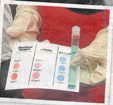
Looking at water quality: Students measuring the sample of water from the river against a scientific chart (inset).
