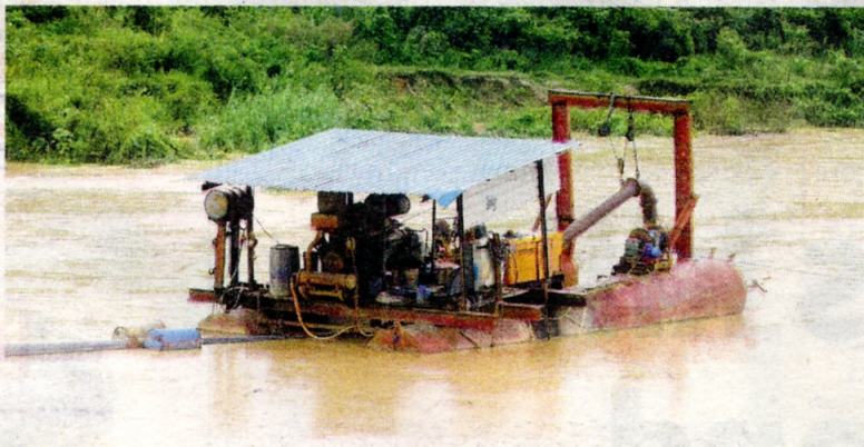
Sand stealer: The pontoon with suction pump which was used to extract sand.
